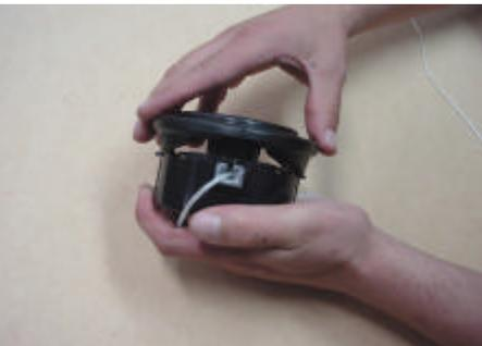
Hold the cord back and line the tabs on the body up with the holes on the cover.
