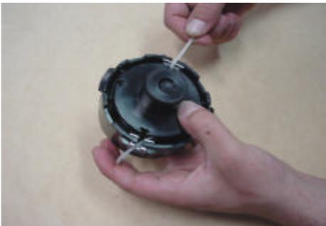
Pull the cord out of the cut outs and bring them back into the eyelets.
