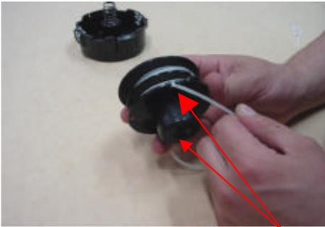
Lock loose ends into the **cut outs** on the front of the spool.
