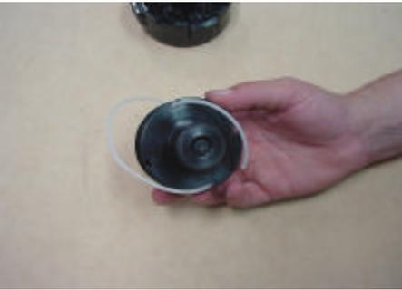
With the spool refilled and the ends of the cord locked into the cut outs in the spool, check that the spring is correctly positioned in the cutter head body.
