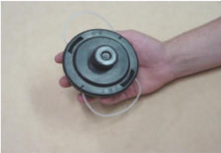
Turn machine off and clean excess grass and dirt from head.
