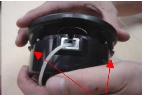
Lightly push in the **tabs** to assemble.
